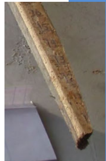
Figure 8.3: Tank gauging stick with broken end (EPA)
