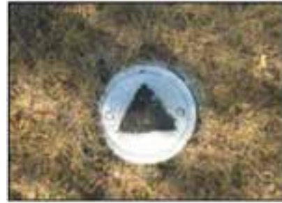
Figure 9.11: Groundwater monitoring well
