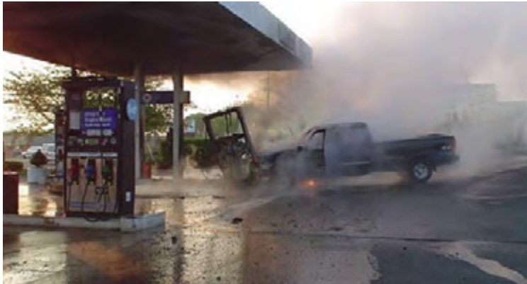
Figure 12.13: Accident where the shear valve failed to shut off fuel flow.
