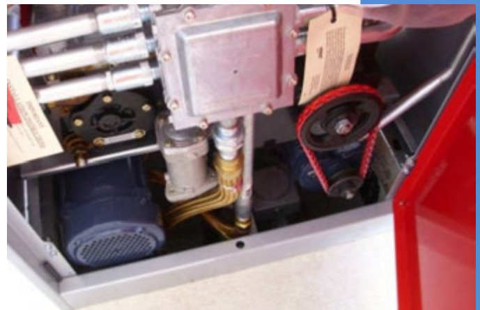
Figure 10.14: Suction system dispenser
