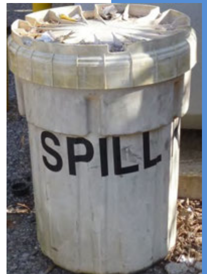
Figure 14.6: Your spill kit should contain absorbent pads or Speedi-dri which can be used to clean up minor spills
