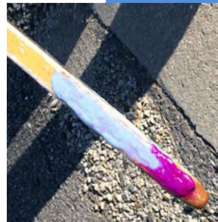
Figure 8.7: Tank gauging stick with water-finding paste. This brand turns red to indicated water level in the tank. Other brands of paste may use different colors.
